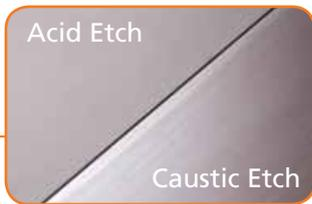
Acid etching is performed in the pre-treatment cleaning process prior to anodizing, replacing the typical caustic etching process. Acid etching better smooths surface imperfections such as extrusion lines and scratches, producing a more uniform appearance as well as changing the bright surface to a matt finish.
